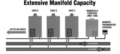
Up to 20 of the Heavy Duty Tankless units can be linked in a manifold configuration to meet the hot water needs of larger applications.
